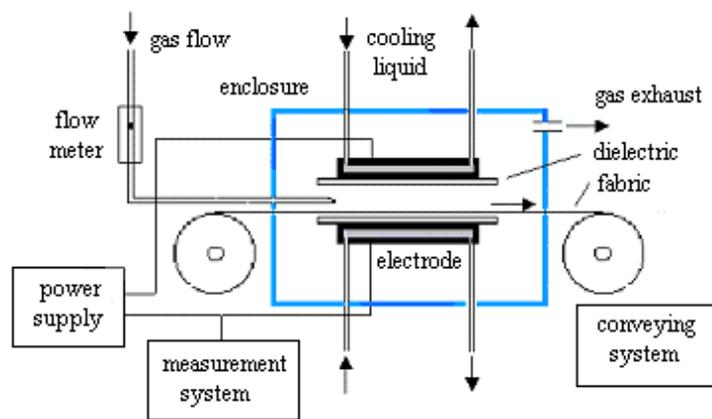
Figure 1. The continuous modification treatment system of dielectric barrier discharge
