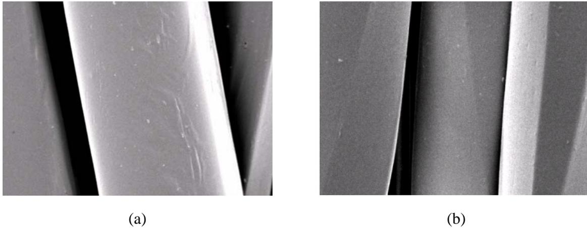
Figure 4. SEM image of untreated polyester fibre. (a) untreated (b) treated
