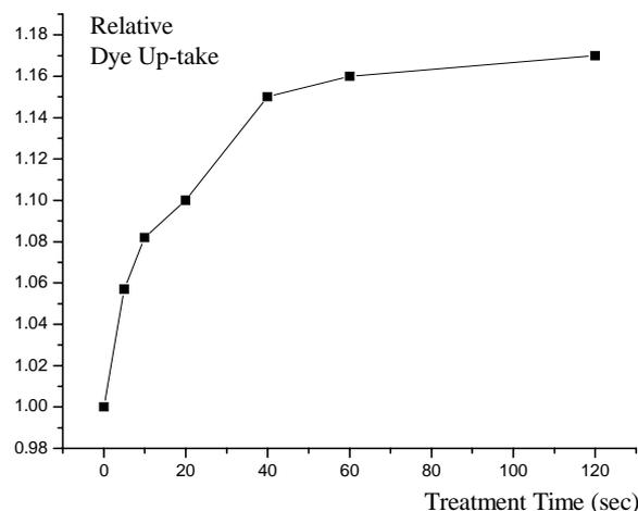
Figure 3. Relative dye up-take versus treatment time
