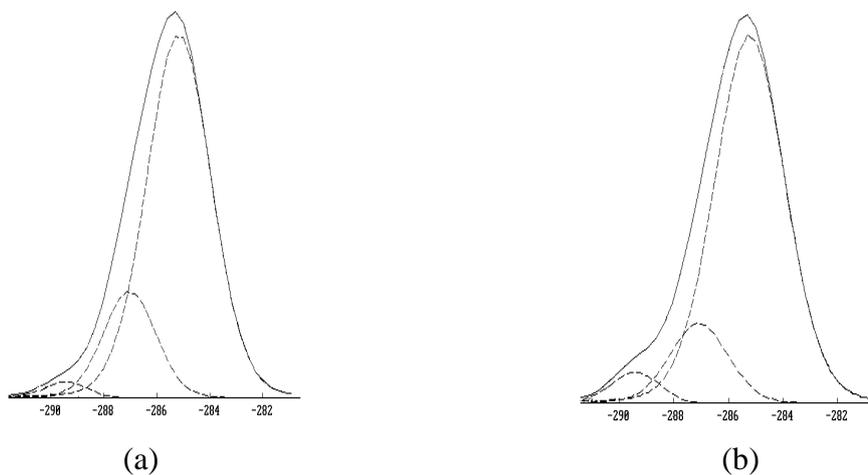
Figure 5. C1s XPS spectra of polyester. (a) untreated (b) treated
