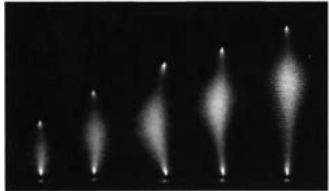
Fig. 2. Photographs of the air glow discharges with various gap lengths ranging from 0.5 to 2 cm. The current was kept constant at 13 mA. The striations in the photographs are due to the limited resolution of the CCD camera.
