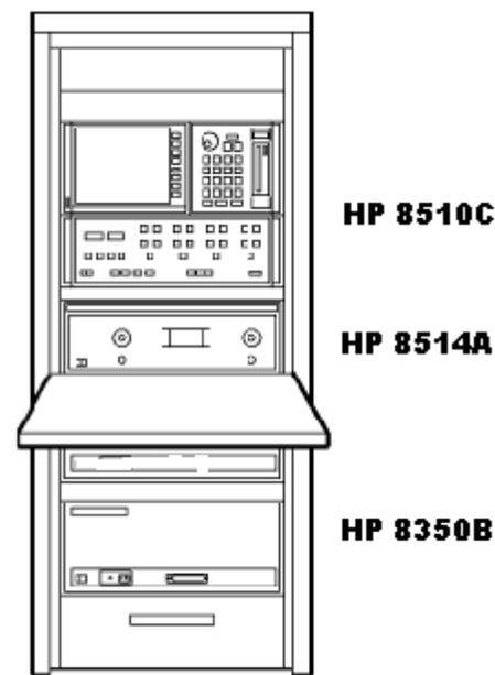
Figure 4: Network Analyzer
