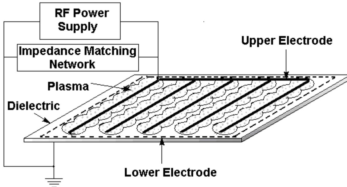
Figure 2: Flat panel reactor
